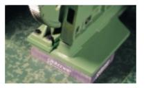
Weaving machine support leg: a layer of Sylomer® under the legs of the equipment reduce the transmission of vibrations into the floor.
