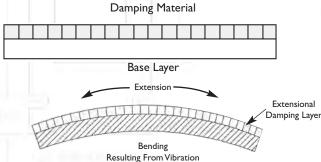
**Above:** a free-layer damping application. This is the most common and most easily installed form of damping. The vibration energy is dissipated through the extension and compression of the damping material due to the vibratory stress of the base layer.
