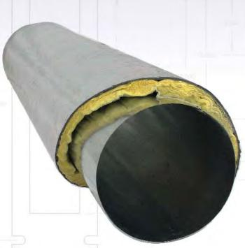
Soundown's QuietLag, acoustic pipe and duct wrap material consists of a fiberglass decoupling layer and TuffMass barrier with reinforced facing. By decoupling the barrier from the pipe or duct this product will greatly reduce noise radiated from plumbing, HVAC ducting and a range of other sources. This wrap will provide effective reduction of breakthrough noise in most pipe and duct applications.
