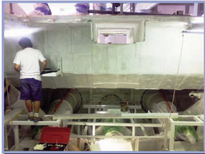
Engine room on yacht – insulated by PROMAGUARD®
