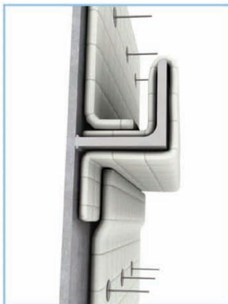
PROMAGUARD® th. 6mm on stiffeners + PROMAGUARD® th. 10mm on steel plate + glass cloth 220gr/m 2 - Contact solution
