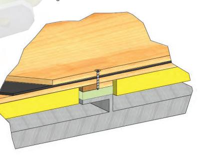
Typical installation of a floated sole on R-12 over a stiffened tank top.
