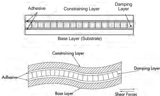
**Above:** a constrained-layer damping application. During vibrational distortion the system flexes creating shear forces on the constraining layer. It is these shear forces that causes the energy to dissipate and turn into heat.
