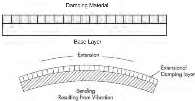
**Above:** a free-layer damping application. This is the most common and easiest form of damping. The vibrational energy is dissipated due to the extension and compression of the damping material due to the vibrational stress of the base layer.
